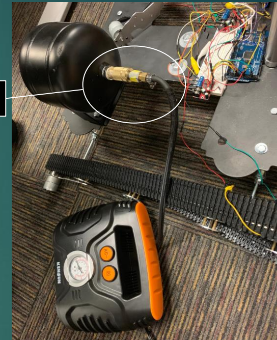
Figure 15: connection between compressor and air tank
